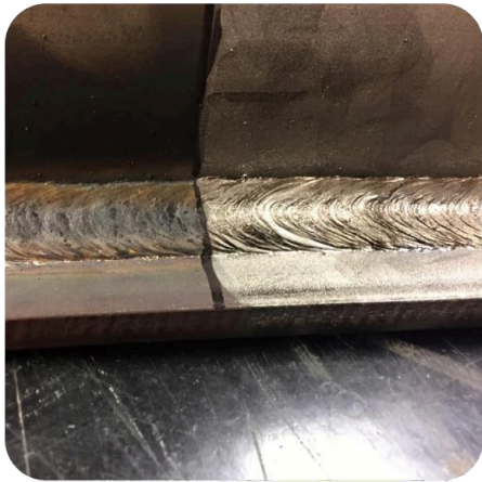
Before and after welding cleaning
