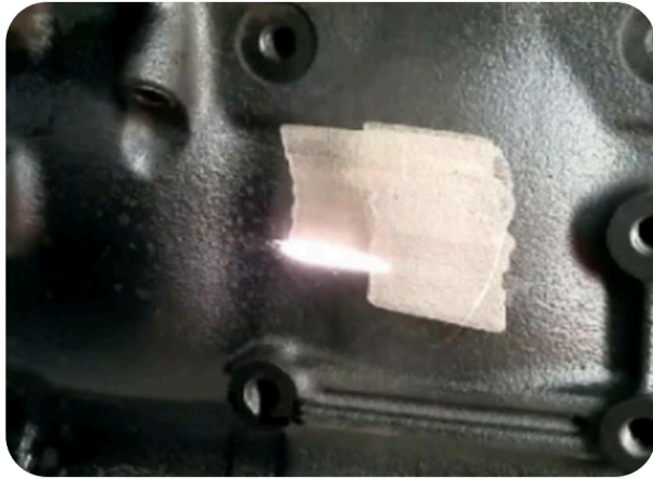
Laser paint removal of auto part
