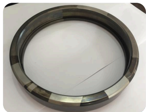
Bearing laser degreasing
