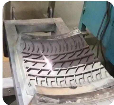
Tire mold cleaning
