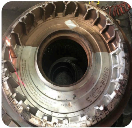
Chrome-plated mold cleaning
