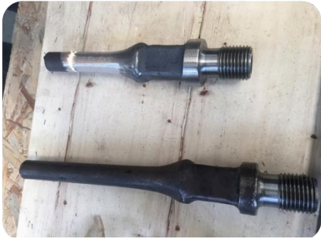
Sucker rod degreasing
