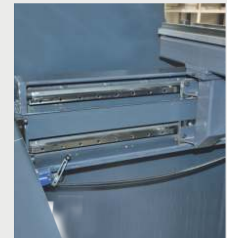
Linear Guided Stronger Back Gauge X Movement
