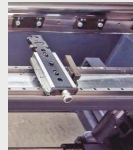
Double Linear Guided Stronger Back Gauges
