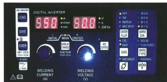
Figure 2 : one knob switch to wire speed display
