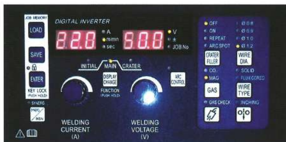
Figure 1 : Current and Voltage Setting (precise to 1A and 0.1V)
